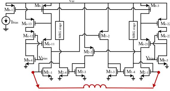
Fig. 9. Circuit implementation of proposed FAI
