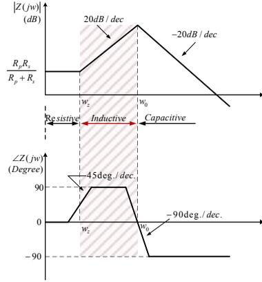
Fig. 5. Bode plots of the impedance of lossy Gyrator-C AI
