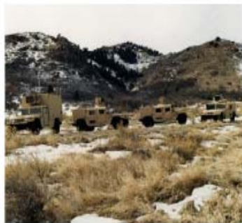
Fig. 1. A team of four robotic scout vehicles manufactured for DARPA's Demo II project. The formation techniques reported in this article were implemented on these robots. Photograph courtesy of Lockheed-Martin.
