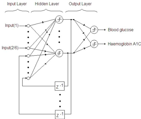
**Fig. 4.** Implementation of Elman neural network for blood glucose and haemoglobin A1C detection
