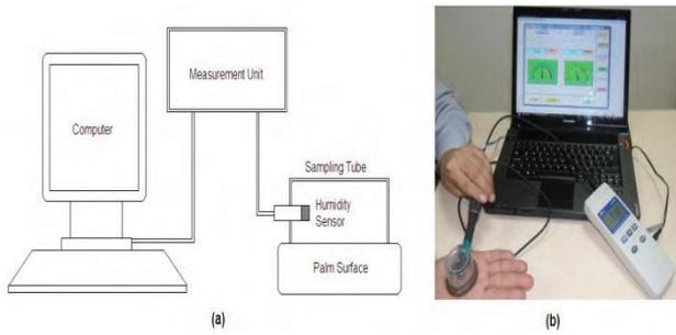
**Fig. 1.** Schematic diagram (a) and a photo view (b) of the measurement system
