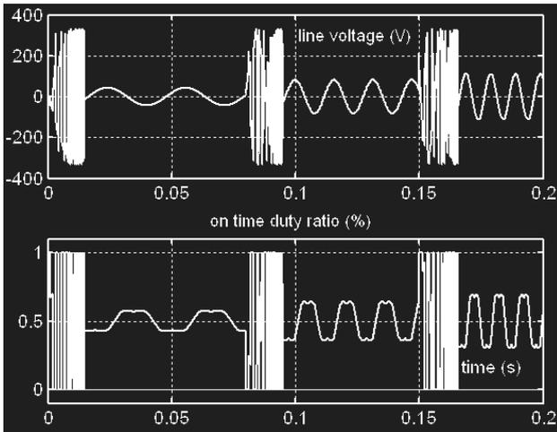
Figure 8: Inverter response to a speed profile
