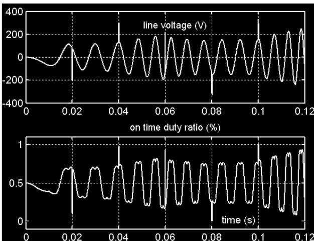
Figure 9: Inverter response to a torque profile
