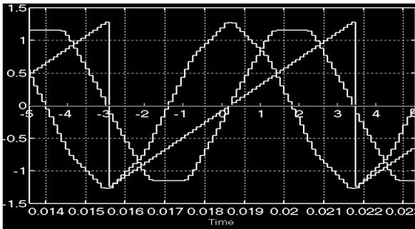
Figure 4: Simulated reference space vector in over modulation
