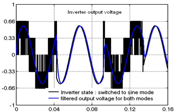
Figure 5: Commutation of the inverter from the switched to sine mode
