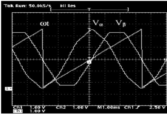
Figure 3: Reference Vector in full modulation
