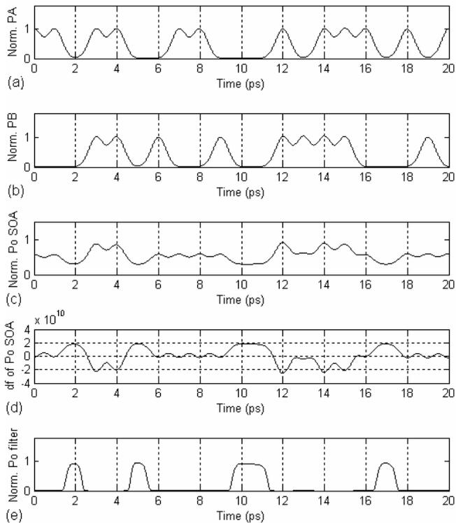
**Fig. 4.** Simulation results for 1ps pulse width (1Tbps). (a) Input power of port A. (b) Input power of port B. (c) Normalized power of SOA output. (d) Frequency shifting of SOA output. (e) Normalized power of optical filter
