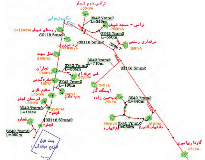
Fig3. The chosen distribution network for implementation of proposed method
