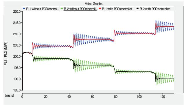
**Fig.6** Variation of PL1 and PL2 when the DSSCs are entered to lines with and without POD controller
