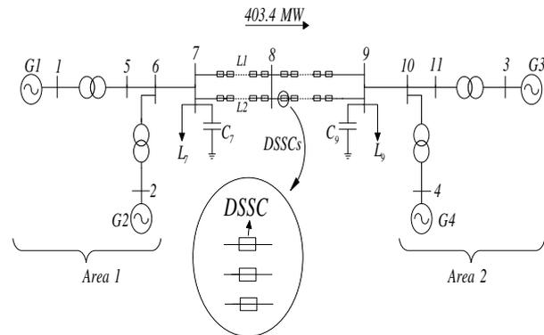
Fig.3 Multi-machine system with DSSC modules in each phase of lines L1 and L2
