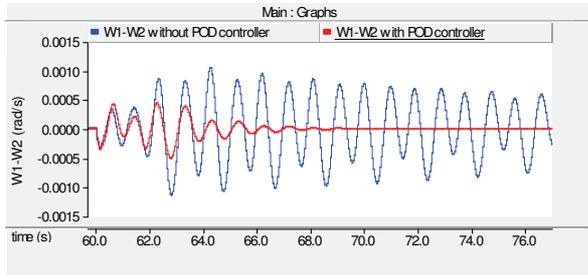
Fig.7 local oscillation mode with and without POD controller
