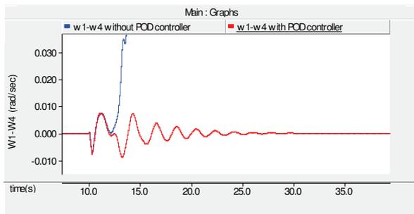
Fig. 9 Inter-area oscillation mode with and without POD controller with severe fault
