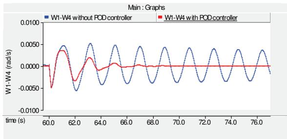
Fig. 8 Inter-area oscillation mode with and without POD controller
