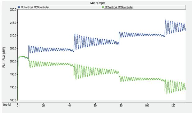
**Fig.4** Variation of PL1 and PL2 when the DSSCs are entered to lines without POD controller
