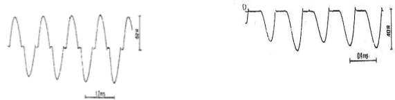
Fig.(3.3): current of the main branch of inverter / I_F / fig.(3.4): current feed / I_Z
