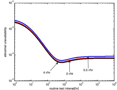
Fig.5. Line repair rate effect on dependability
