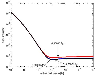
Fig. 13 Breaker inadvertent opening rate effect on security
