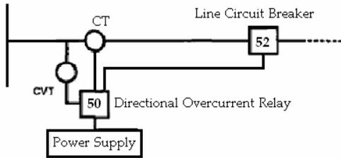
Fig.2 Overcurrent system protection of a feeder
