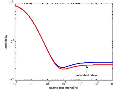
Fig. 16: Relay redundancy effect on reliability
