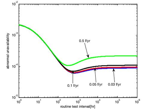
Fig.6. PSU failure rate effect on dependability
