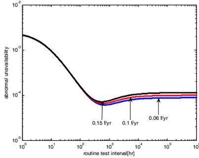
Fig. 12: Breaker failure rate effect on dependability
