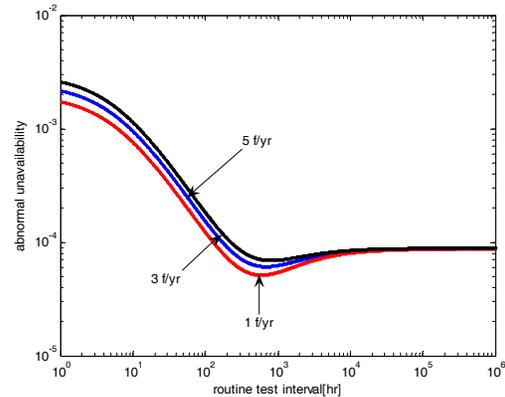
Fig.3. Line Permanent failure rate effect on dependability
