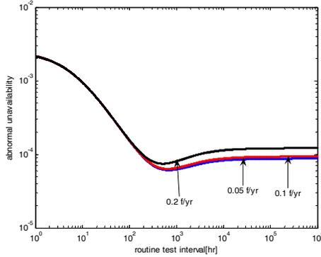
Fig.7. CT failure rate effect on dependability
