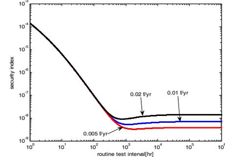
Fig.10: Relay potential mal-trip effect on security
