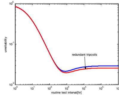
Fig. 17: Trip Coil redundancy effect on reliability
