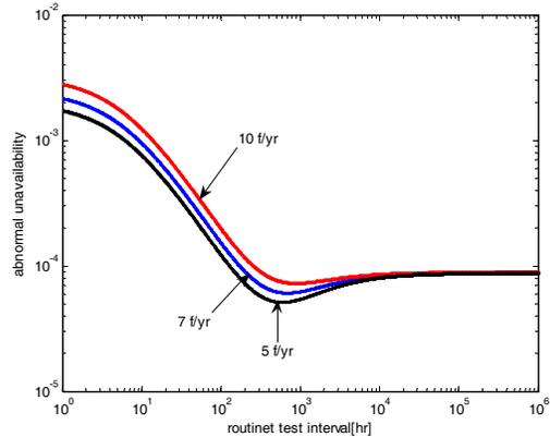
Fig.4: Line temporary failure rate effect on dependability
