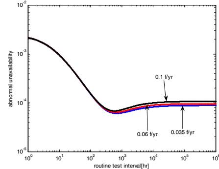
Fig.11: Trip coil failure rate effect on dependability
