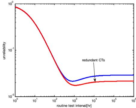
Fig. 14: CT redundancy effect on reliability
