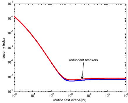
Fig.18: Breaker redundancy effect on security
