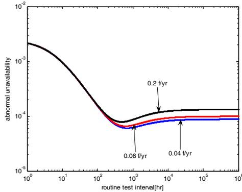
Fig.8: VT failure rate effect on dependability
