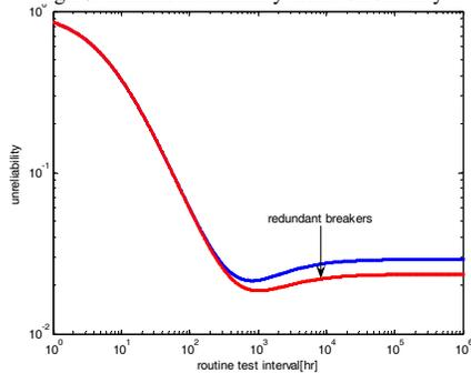
Fig.19: Breaker redundancy effect on reliability
