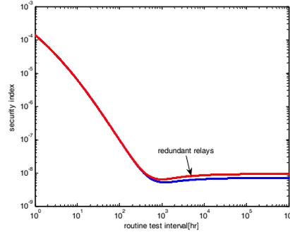
Fig. 15: Relay redundancy effect on security
