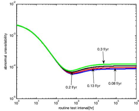
Fig.9: Relay failure rate effect on dependability
