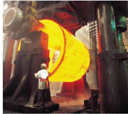
SHELL FORGING - 10,000/ 13,000 ton Forging Press DOOSAN-KORE: Dövme İmalat
