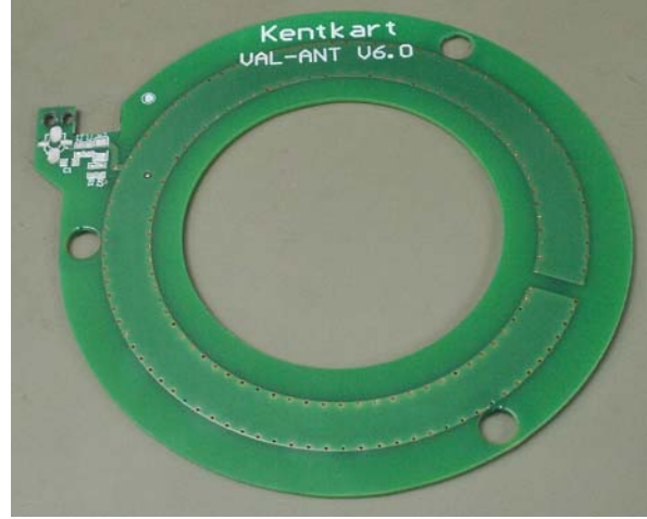
Fig. 4. The designed PCB antenna
