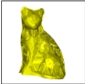
Figure 4 - 3D Delaunay Mesh l_2 alpha = 0.061, removed interior vertex number = 1304, removed boundary vertex number = 491
