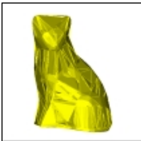
Figure 5 - 3D Delaunay Mesh l_3 alpha = 0.098, removed interior vertex number = 810, removed boundary vertex number = 305
