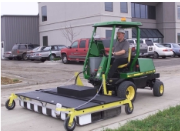
Fig. 5 Tractor driven CART GPiR system.
