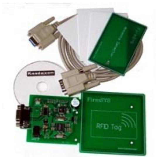
Picture 1: rfid starter kit QB-RFIDKIT
