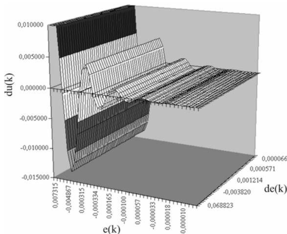
Fig. 10. Hyper Plane of the output signal  $\Delta u$  versus error inputs  $e$  and  $\Delta e$ .
