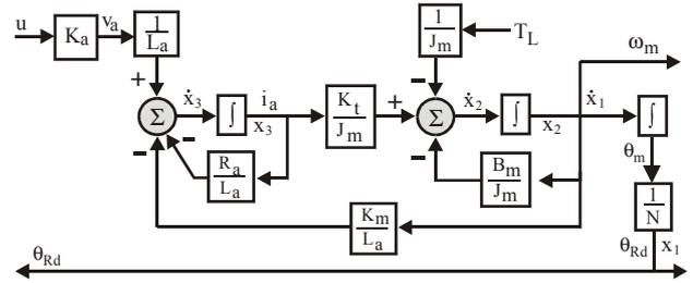
Figure 5. Simulation Diagram for PMDC Motor and gear system.
