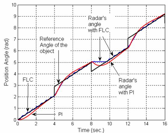
Figure 8. Radar tracking performances of both FL and PID controllers.
