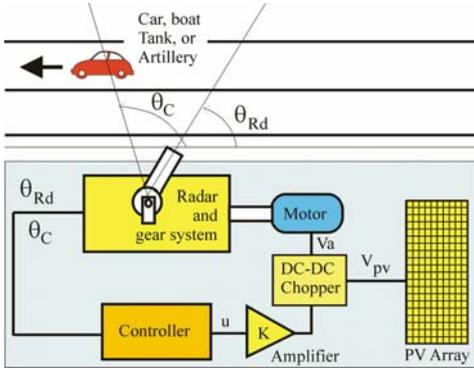
Figure 1. Schematic diagram of the tracking control system
