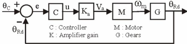
Figure 4. General block diagram of the Unified Motor-Control System.
