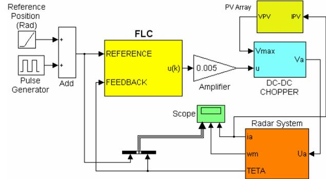
Figure 7. Fuzzy Logic FLC Control Scheme Using the PMDC motor for Radar Detection
