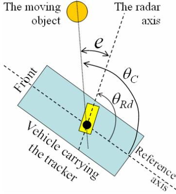
Figure 3. The schematic diagram of the tracking system.
