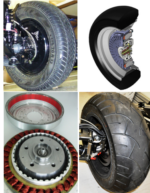
Figure 2. EOsc cars BLDC motors. Top left: Non modified electric scooter BLDC motor used on EOsc1. Top right: CAD design of modified electric scooter BLDC motor for use on EOsc2. Bottom left: Modified rotor and stator parts of BLDC motor. Bottom right: Modified BLDC motor on EOsc2.
