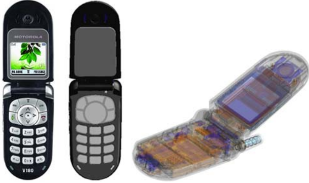
Figure 1. Multiband phone used in this study: photograph of the actual phone (left) and the CAD derived model
