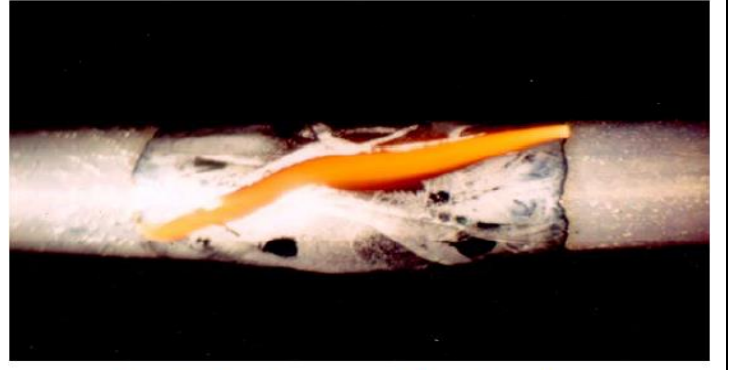
Fig. 2. The Cu_2O breeding process (Photo: Yasuaki Hagimoto).
