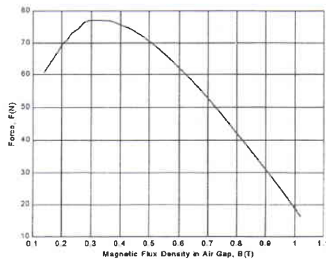
Figure 5. Force versus air gap flux density.
