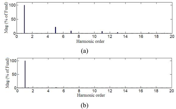
**Fig. 6.** Frequency spectrum of the load and source current: (a) For load current. (b) For source current.
