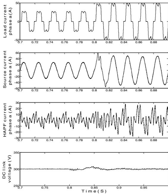
**Fig. 8.** Simulation results of HAPF under the step load change
