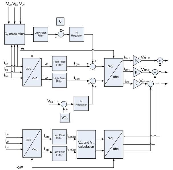
Fig. 4. Proposed control scheme block diagram
