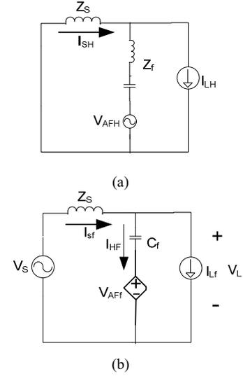
Fig. 3. Single-phase equivalent circuit of the HAPF. (a) For current harmonic compensation. (b) For reactive power compensation
