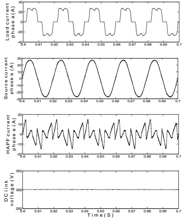
**Fig. 5.** Simulation results of HAPF with proposed control method
