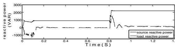
**Fig. 9.** Source and load reactive power under the step load change
