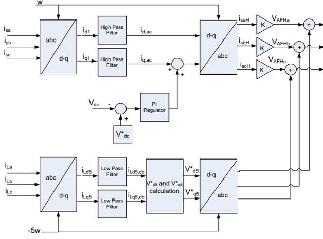
Fig. 2. Conventional control scheme block diagram
