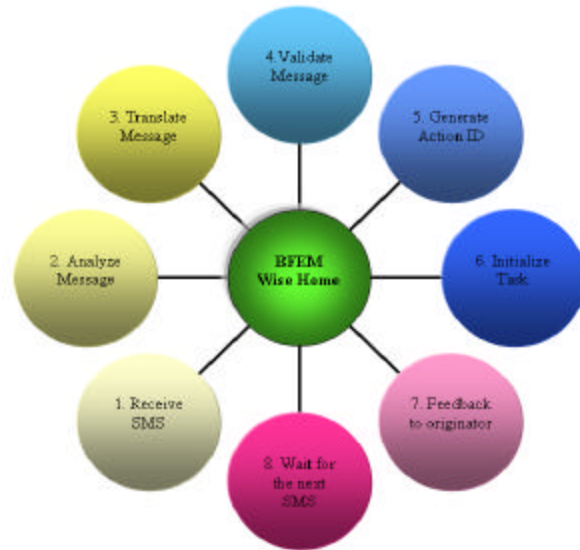
Figure IV.1 (Home/factory automation process flow diagram)
