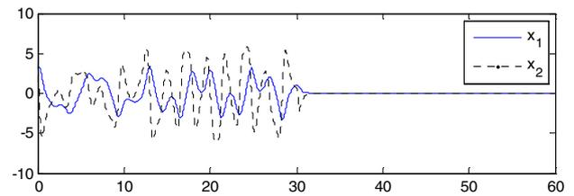
Fig. 4: The time responses of the state variables of the Duffing's oscillator with control activated at  $t = 30$ .
