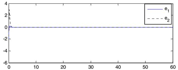
Fig. 3: The time responses of the observer error vectors for  $u=0$ .
