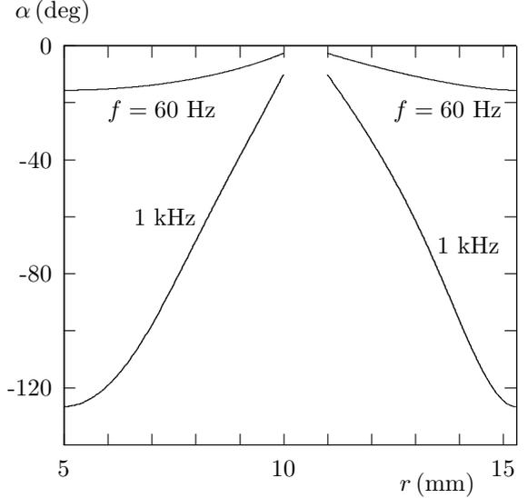
Figure 2. Initial phase angle  $\alpha(r)$  of the current density in conductors.
