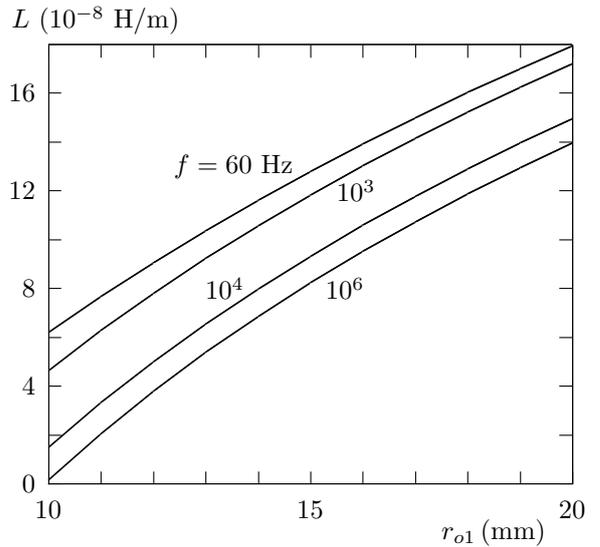
Figure 3. Dependence of inductance  $L$  on  $f$  and  $r_{o1}$ , calculated using formula (11).
