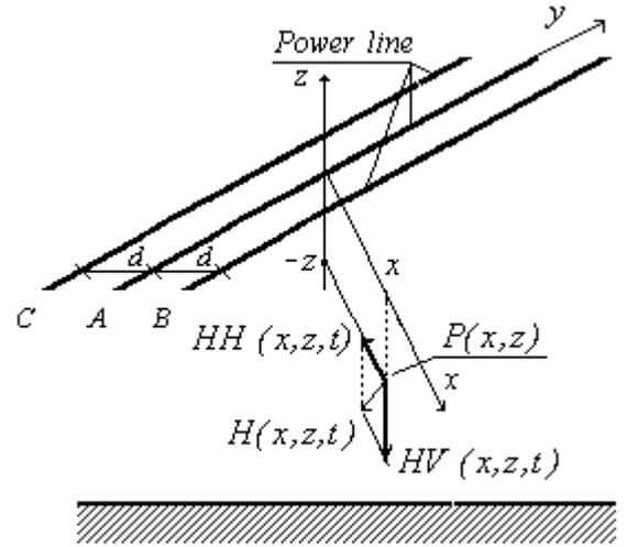
Fig. 1. Schematic illustration of the three-phase power line.
