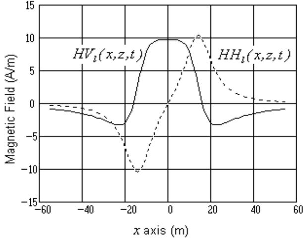
Fig. 4. Vertical ( $HV_1(x,z,t)$ ) and horizontal ( $HH_1(x,z,t)$ ) components generated by the loop 1-2-3-4 ( $i(t)=565\sin\omega t$  A,  $d=14$  m,  $z=-15$  m,  $h=7$  m,  $t=0$ ).
