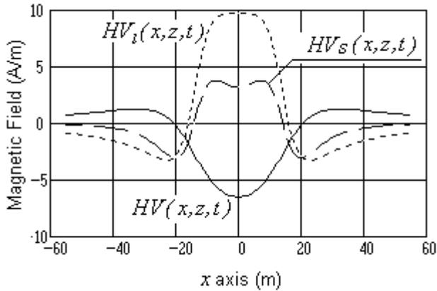
Fig. 5. Vertical components of three-phase line ( $HV(x,z,t)$ ), of the loop ( $HV_1(x,z,t)$ ) and their difference ( $HV_s(x,z,t)$ ) as function of  $x$ .
