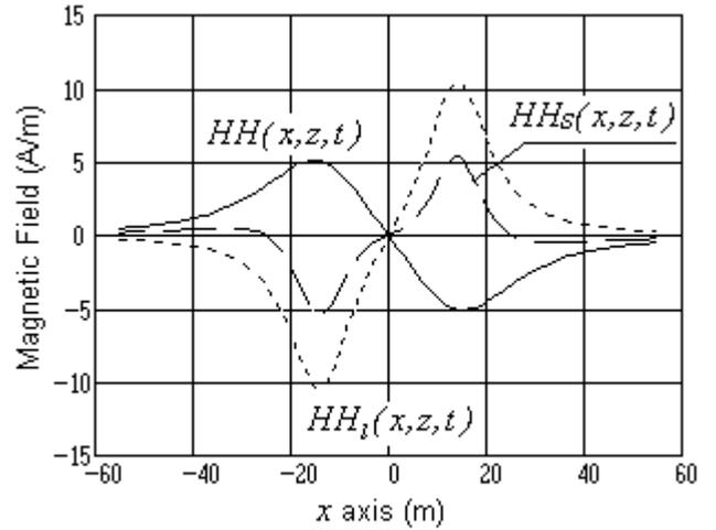
Fig. 7. Horizontal components of three-phase line ( $HH(x,z,t)$ ), of the loop ( $HH_1(x,z,t)$ ) and their difference ( $HH_s(x,z,t)$ ) as function of  $x$ .
