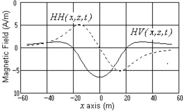
Fig. 2. Vertical ( $HV(x,z,t)$ ) and horizontal ( $HH(x,z,t)$ ) components, generated by the three-phase power line ( $i(t)=700\sin\omega t$  A,  $d=14$  m,  $z=-15$  m,  $t=0$ ).
