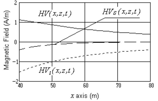
Fig. 6. Vertical components of three-phase line ( $HV(x,z,t)$ ), of the loop ( $HV_1(x,z,t)$ ) and their difference ( $HV_s(x,z,t)$ ) as function of  $x$ .
