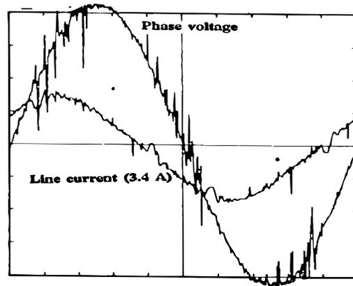
Figure 5b: Sinusoidal i/p voltage and line current at leading power factor,  $M = 0.8$  (experimental) SW/div, 2A/div & 2ms/div
