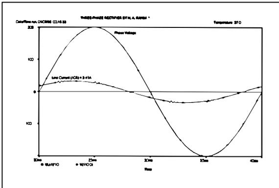
Figure 5a: Sinusoidal input voltage & current at leading p.f (simulated)
