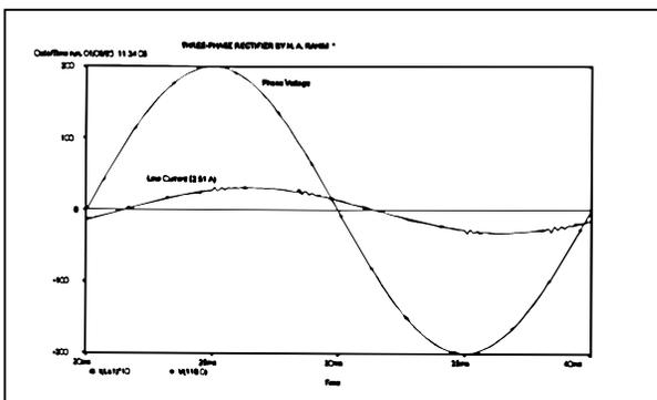
Figure 6a: Sinusoidal input voltage & current at lagging p.f (simulated)
