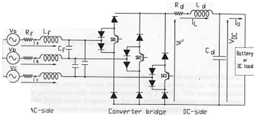
The voltage produced by the bridge,  $V_L$  is low-pass filtered by an  $L_d C_d$  combination to provide an output voltage  $V_{DC}$ . The converter is operated as a step-down converter where the output voltage can be controlled in the range of 0 to  $1.5 \hat{V}_{ph}$
