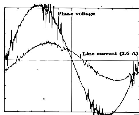
Figure 6b: Sinusoidal i/p voltage and line current at lagging power factor,  $M = 0.8$  (experimental)
