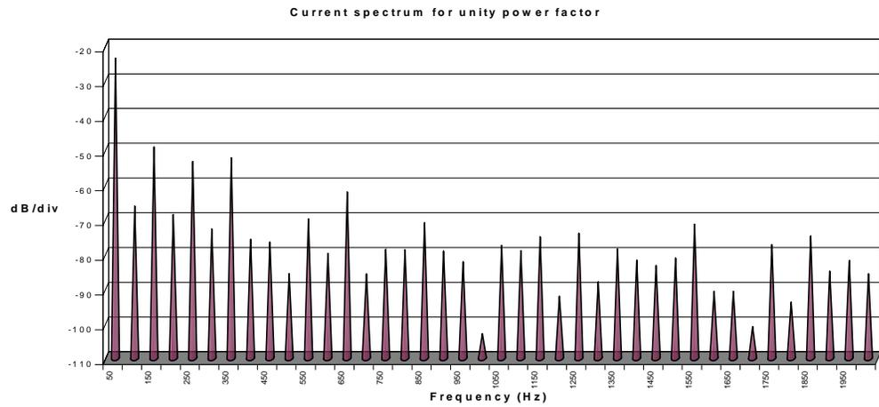
**Figure 7: Line current spectrum at unity power factor**
