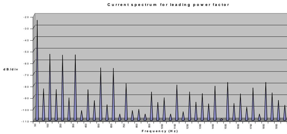
**Figure 8: Line current spectrum at leading power factor**
