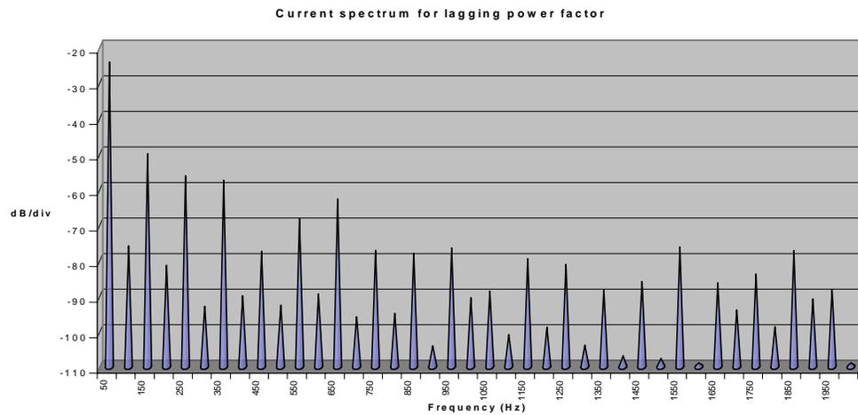
**Figure 9: Line current spectrum at lagging power factor**
