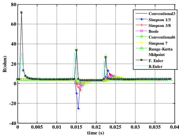
Fig. 2. Not filtered R values calculated before and after the fault
