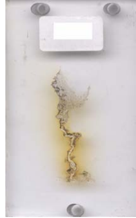
Figure 1: Surface tracking patterns of some polyester samples obtained ASTM D 2303 Inclined Planed Tracking Test
