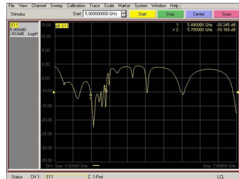
Fig.3. Reflection coefficient-S11 of waveguides that are loaded different length inclusions a. 6cm-10 TSSRRs b. 7cm-11TSSRRs c. 7.5cm-12 TSSRRs d. 8cm-13TSSRRs
