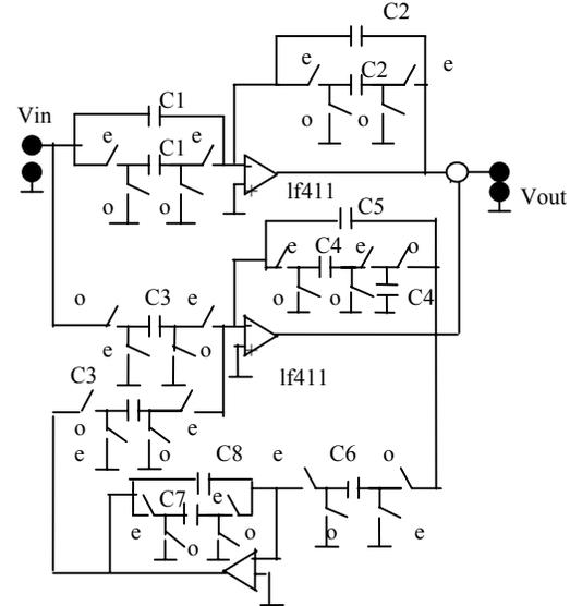
Fig 2: Second Order Schneider Based SC Half Differentiator
