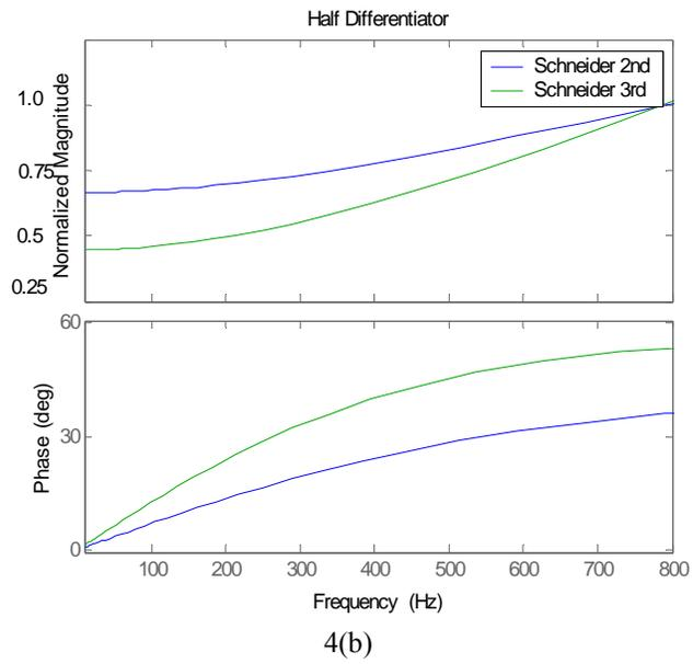
Fig 4: Simulation Results of Schneider Based Second and Third Order Half Differentiator using (a) OrCAD Pspice and (b) MATLAB.
