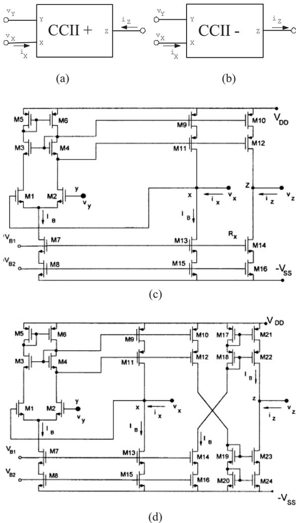
**Fig. 8.** (a) Circuit representation of an ideal CCII+; (b) circuit representation of an ideal CCII- CMOS realization of an CCII+ and (d) CMOS realization of an CCII- [7]
