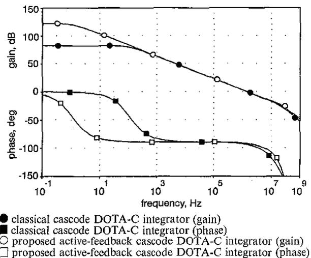
Fig. 7. Gain and phase response of simulated DOTA-C integrators [4]
