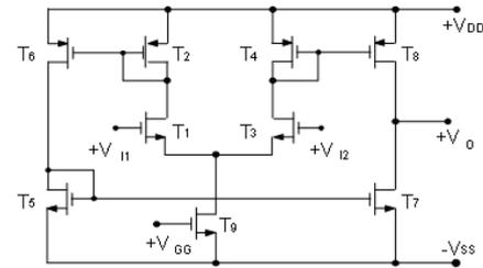
Fig. 3. Simple symmetrical CMOS OTA structure.
