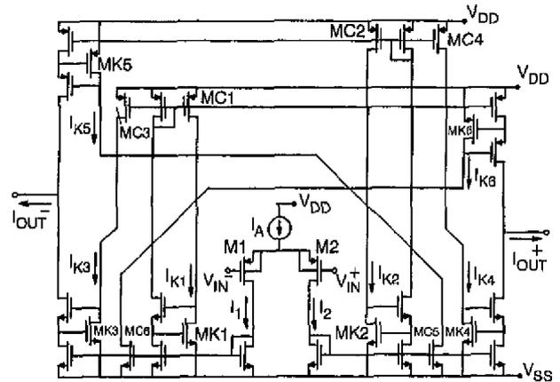
Fig. 6. Proposed CMOS DOTA structure [4]
