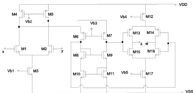
Fig. 12. CMOS realization of FTFN [9].
