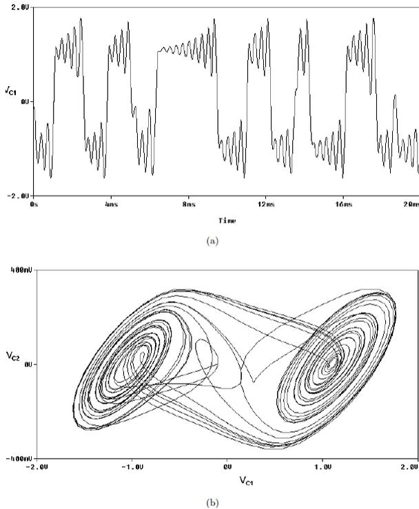
**Fig. 15.** When improved mixed-mode chaotic circuit oscillates in autonomous mode (S1-OFF, S2-ON), (a) the chaotic waveform of the voltage across capacitor C1 in Fig. 13, and (b) double-scroll chaotic attractor.
