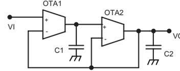
Fig. 2. LP filter derived from Fig.1b.
