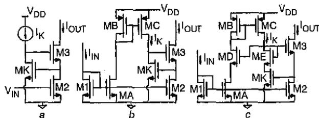
Fig. 5. Active-feedback cascode structures a) RGC surge b) Active-feedback cascode CM c) Improved active-feedback cascode CM [4]
