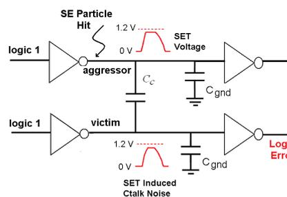
Fig. 1. SE crosstalk noise (lumped wire model is for demonstration).
