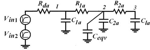
**Fig. 6.** Decoupled aggressor line for coupling node voltage calculation.
