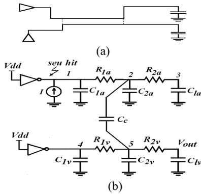
Fig. 2. The 4- $\pi$  model for two coupled interconnects
