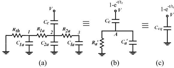
**Fig. 4.** A non-switching aggressor net coupled to the victim line
