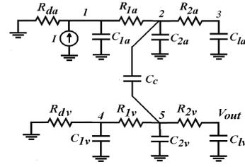
Fig. 3. SE crosstalk calculation using the 4- $\pi$  template circuit.
