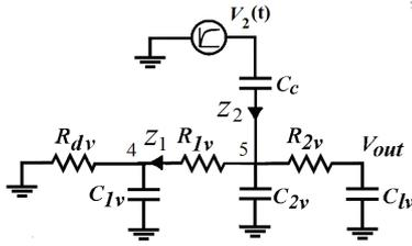
Fig. 8. Output voltage calculation.
