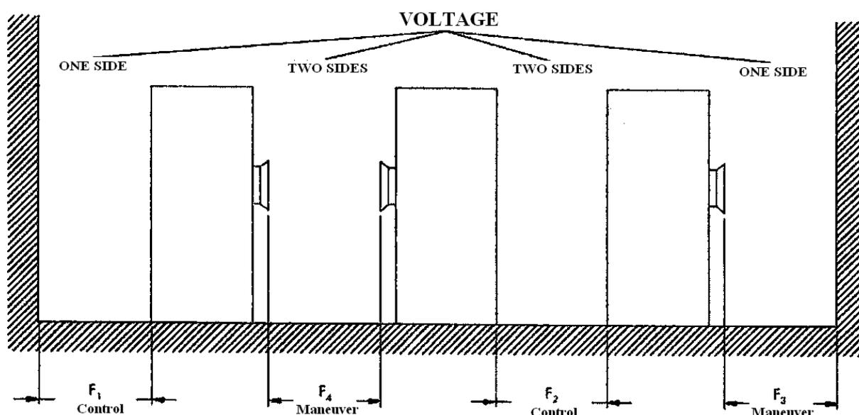
*Figure 1: Passage widths when the cubicle faces are wire cage door and solid wall*
