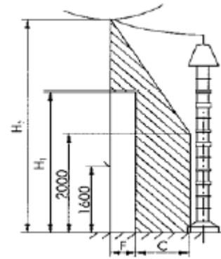
*Figure-7 Protection area of the devices placed on earth and having normal fence with passage.*
