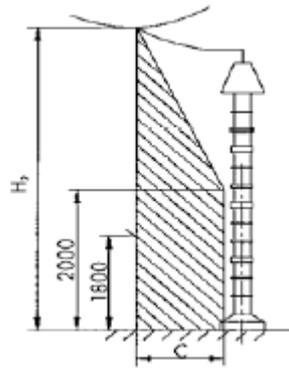
*Figure-6 Protection area of the devices placed on earth and having normal fence without passage*
