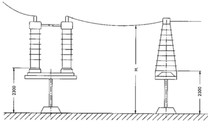
Figure – 3: The heights of the conductors on the surfaces for walking, not surrounded with fence in the installation (in accordance with Table 3).
