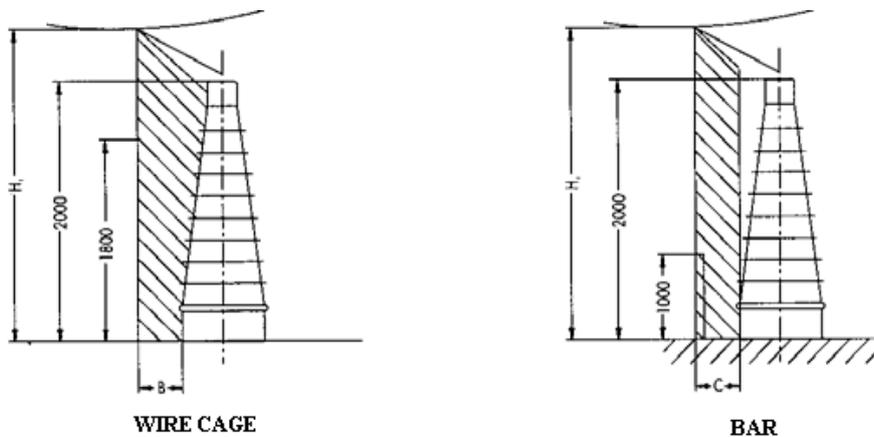
Figure 4- Protection area and minimum height ( $H_1$ ) in the installation
