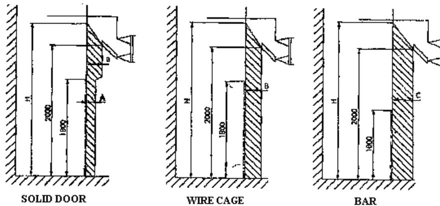
Figure – 2 Protection areas (shaded sections) and minimum heights in open connection installations. The values on the figure are valid only up to 30 kV. See Figure 4 for voltages of 45 kV and higher. The letters above show the clearances in Table 1.
