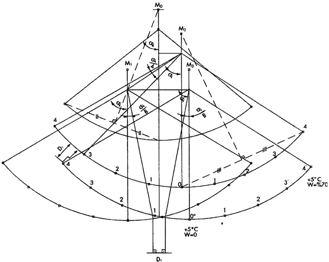
Figure – 8: Conductor oscillation diagram
