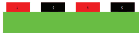
Fig. 6. Detail of a classic translator with surface mount magnets
