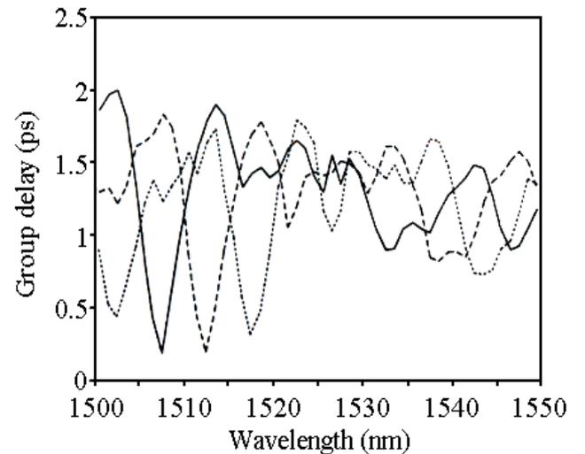
Fig. 2. PMD spectra of a cabled fiber at temperatures of 30°C (solid), 25°C (dashed) and 20°C (dotted)
