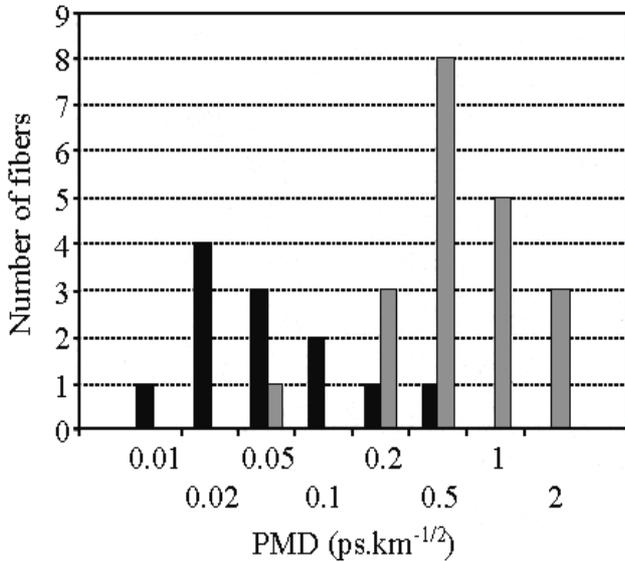
Fig. 1. Measured PMD values of spooled (black bars) and cabled (grey bars) fibers
