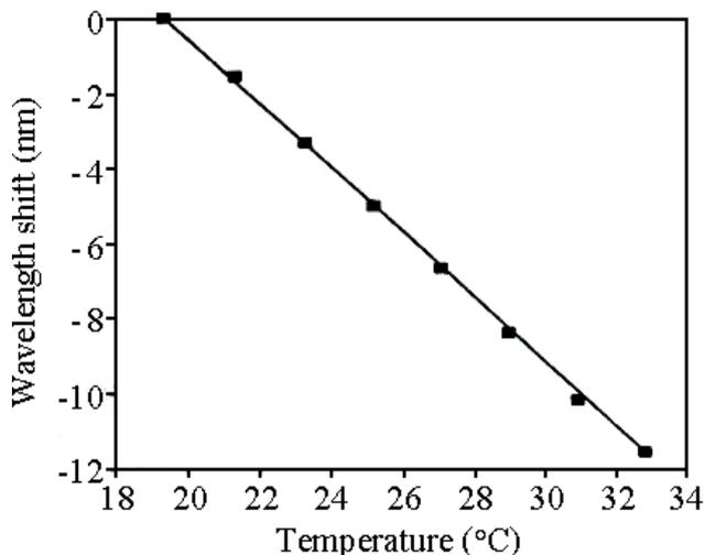
Fig. 3. Shift of the PMD spectrum of a cabled fiber
