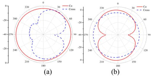
**Fig. 11.** The measured radiation pattern at 2.4GHz (a) y-z plane and (b) x-z plane
