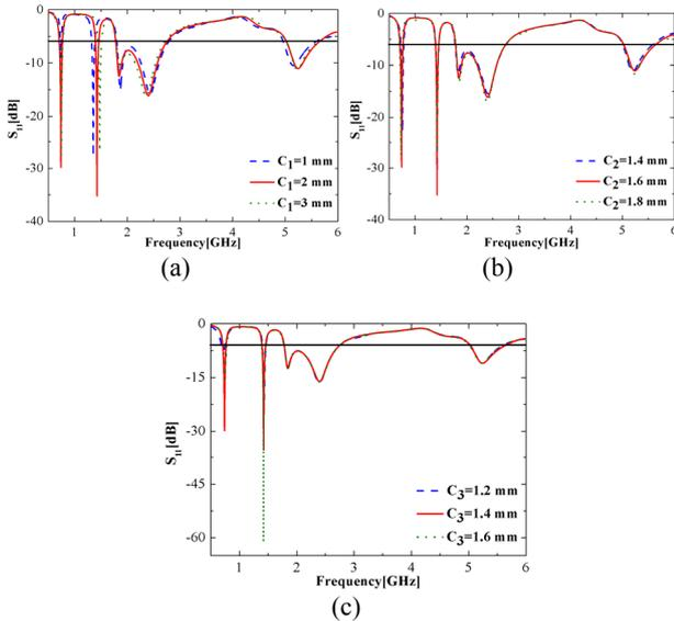
**Fig. 3.** The simulated  $S_{11}$  of meander-line monopole with parameters (a)  $C_1$  (1.5GHz), (b)  $C_2$  (1.9GHz) and (c)  $C_3$  (0.7GHz)
