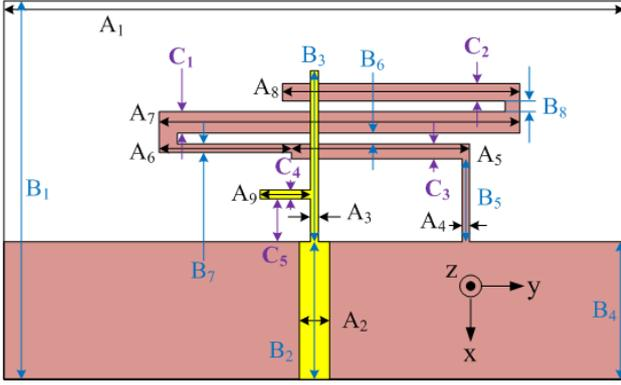
Fig. 1. The antenna geometrical layout and physical parameters
