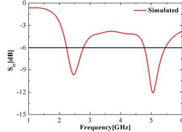
Fig. 2. The simulated S<sub>11</sub> of tree-type monopole
