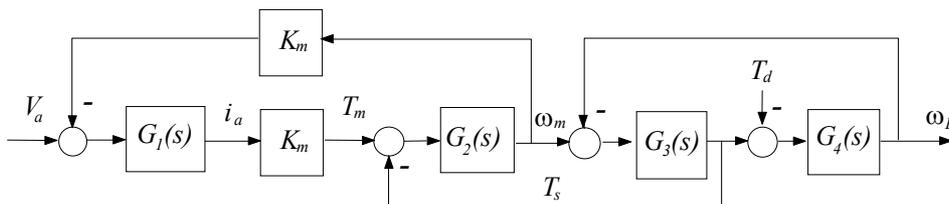
Figure 2. Block diagram of the linear two-mass system.
