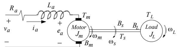
Figure 1. A schematic diagram of the linear two-mass system.
