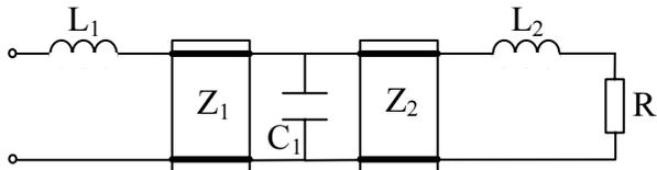
Figure 2. Synthesized low-pass mixed-element network, normalized element values:  $L_1 = 6, L_2 = 4, C_1 = 3, Z_1 = 2, Z_2 = 5, R = 1$ .
