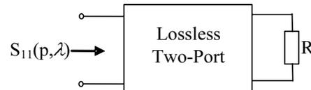
Figure 1. Lossless two-port with input reflectance function  $S_{11}(p, \lambda)$ .
