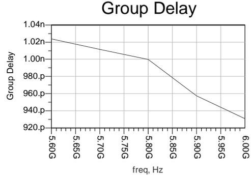
Fig. 3. Delay Characteristic of Used Amplifier
