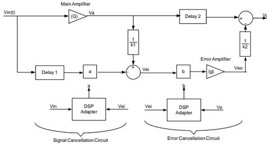
Fig. 2. Adaptive Feedforward Amplifier Model
