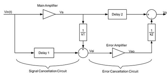
**Fig. 1. General Architecture of Feedforward Amplifier**
