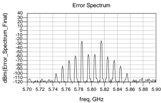
**Fig. 7. Error Signal (Signal Cancellation Output)**
