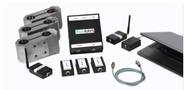
Figure 1: The Developed Force Measurement System
