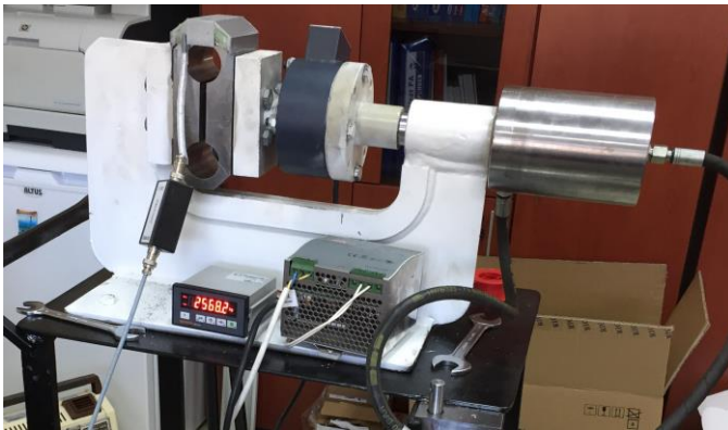
Figure 7: Hydraulic Test Apparatus for Determining Tension and Compression Coefficients
