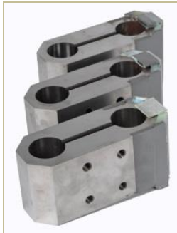
Figure 2: Custom Designed 3D Force Transducers
