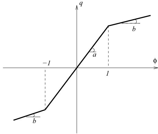
**Figure 3.** Piecewise linear characteristic of a flux-controlled memristor.
