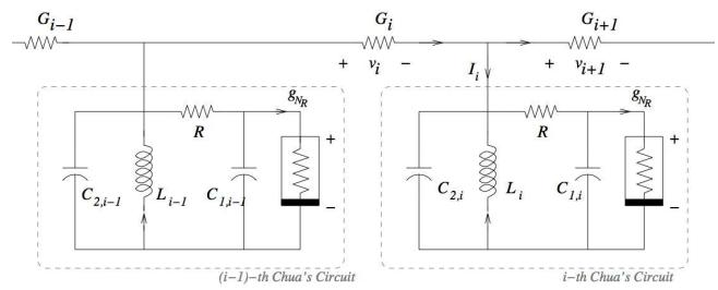
**Figure 1.** One dimensional Cellular Neural/Nonlinear Network circuit consist of Chua's circuits. Each Chua's circuit is coupled with resistor.
