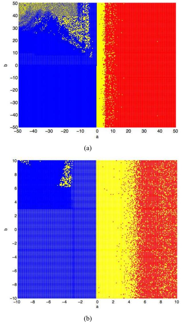
**Figure 5.** The network dynamic due to the parameter space of the memristor. Yellow, red and blue regions denote the regions of synchronous, non-synchronous and unstable behavior, respectively for (a)  $|a| < 10$  and  $|b| < 10$  and (b)  $|a| < 50$  and  $|b| < 50$ .
