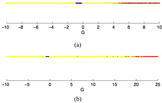
**Figure 2.** The network's dynamic behavior due to the coupling straight. Yellow, red and blue regions denote the regions of synchronous, non-synchronous and unstable behavior, respectively. (a)  $L = 10$  (number of circuits) and (b)  $L = 20$ .
