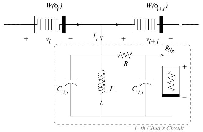
**Figure 4.** A cell of the CNN consist of Chua's circuit. Each cell is coupled to its neighbors with identical flux-controlled memristor.
