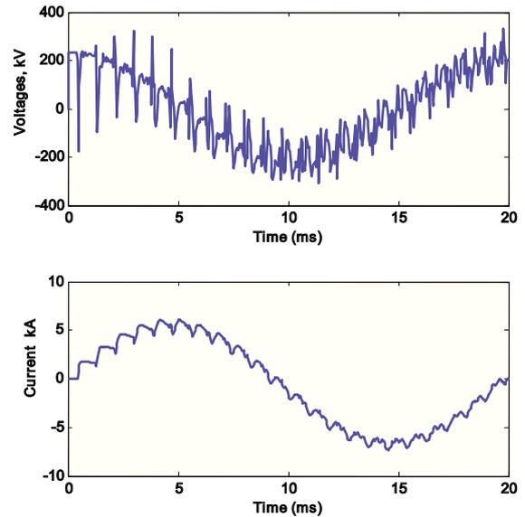
Fig. 2. Transient a) voltage and b) current waveforms for a fault at 120 km from the sending-end.
