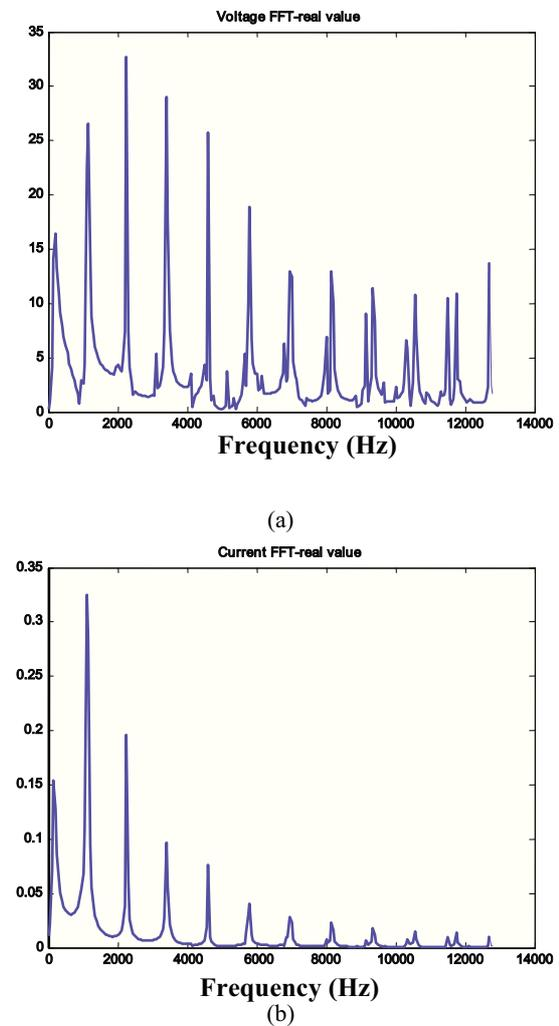
Fig. 3. Transient response in frequency domain; a) voltage, b) current.
