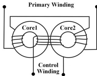
**Fig.4.** Basic structure of the LVI.
