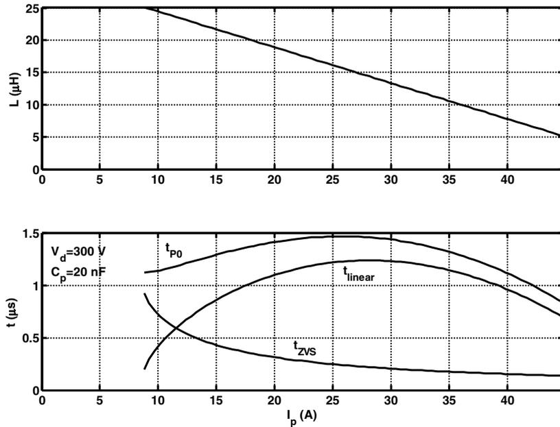
Fig. 3. Lagging leg transition durations according to the LVI variation.
