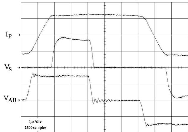
**Fig 6.**  $I_p$  (25A/div),  $V_s$  (100V/div) and  $V_{AB}$  (200V/div) waveforms for  $I_o = 140$  A respectively.
