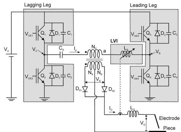
**Fig.1.** LVI controlled PSPWM DC-DC converter for arc welding applications.
