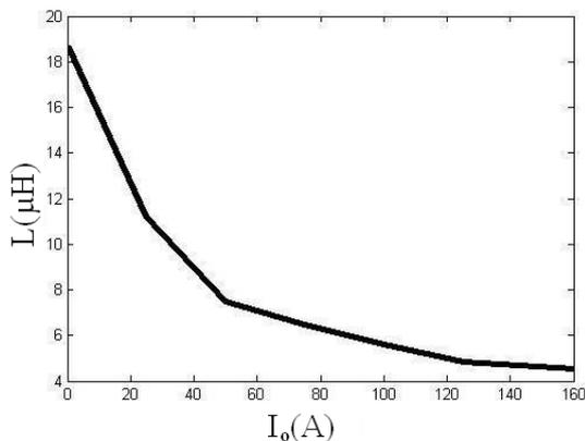
**Fig.5.** Experimental variation of inductance with output current.
