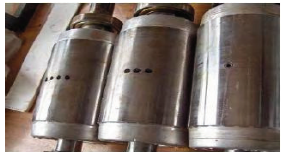
Fig. 4. Rotor with one broken bar.
