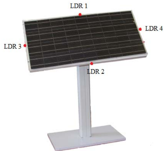
Fig. 5. Mechanical structure of two axis tracker
