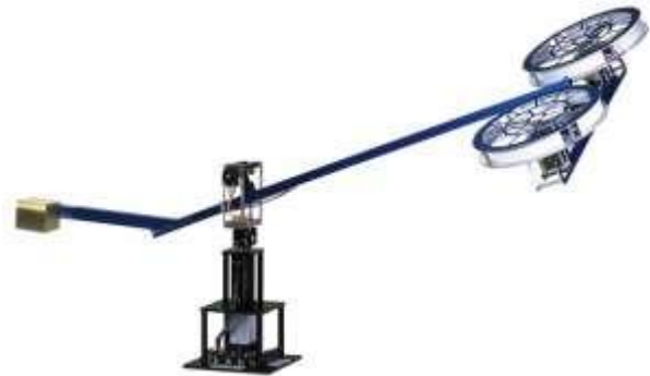
Figure 1. 3-Dof Helicopter System
