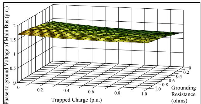
Figure 6. Maximum phase-to-ground overvoltages of phase "a" at the main HV bus, obtaining for the optimum switching instants shown in Figure 4, as a function of the trapped voltage and neutral grounding resistance.
