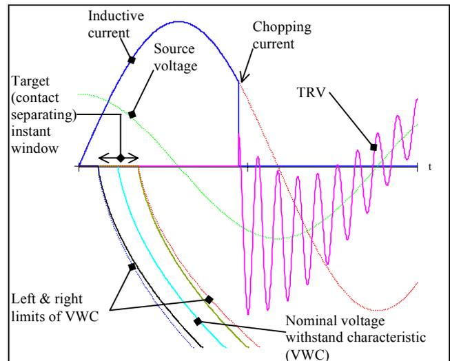
Figure 2. Diagram illustrating the breaking instant window for a case of successful inductive current interruption.
