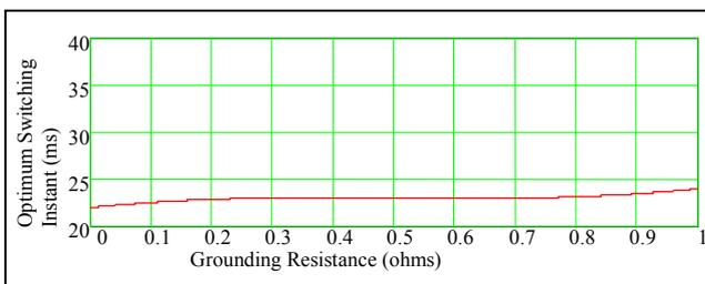
Figure 8. Optimum switching instant for the breaker pole of phase "a", as a function of the neutral grounding resistance.
