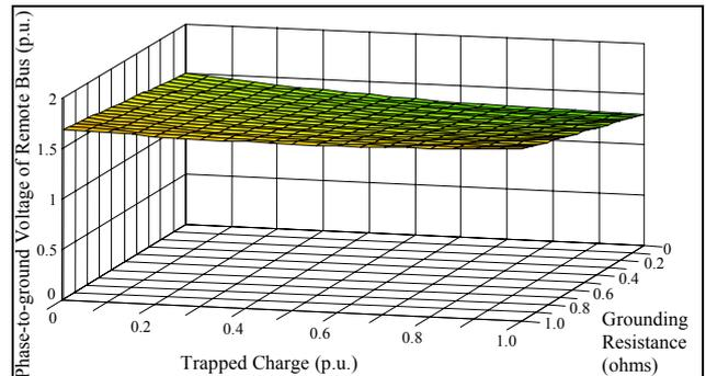
Figure 7. Maximum phase-to-ground overvoltages of phase "a" at a remote bus, obtaining for the optimum switching instants shown in Figure 4, as a function of the trapped voltage and neutral grounding resistance.
