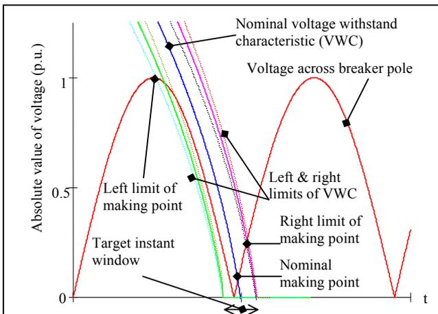
Figure 1. Diagram illustrating the making instant window for a case where target instant corresponds to zero voltage.
