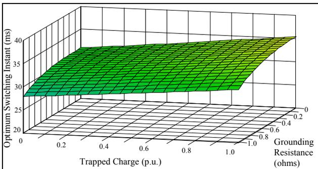
Figure 4. Optimum switching instant for the breaker pole of phase "a", as a function of the trapped voltage and neutral grounding resistance.
