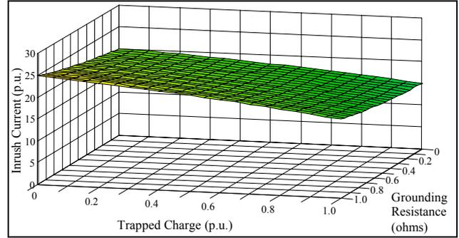
Figure 5. Maximum inrush currents of phase "a", obtaining for the optimum switching instants shown in Figure 4, as a function of the trapped voltage and neutral grounding resistance.
