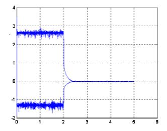
In Figure-3, star connected induction motor stator phase voltages are shown during the implemented automated stator transient inductance measurement algorithm.
