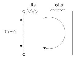
As soon as the rotor flux changes, rotor circuit should be included to the equivalent circuit. But for approximately stator transient time constant duration, current follows the trajectory determined by stator resistance and transient inductance. In the sub-transient region, stator phase current decays from initial dc value to a lower value with a very high rate of decrease. The current response of the stator phases in sub-transient region may be modeled as:
