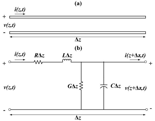
**Fig. 1.** (a) The voltage and current definitions of two-wire transmission line (b) The equivalent lumped-element circuit
