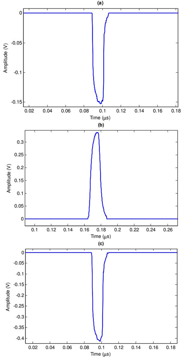
**Fig. 6.** Modified zero-padded waveforms; (a) mismatch reflection, (b) DUT response, and (c) incident pulse
