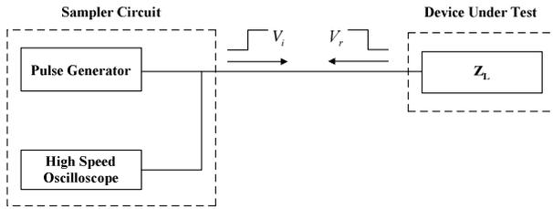
**Fig. 2.** Functional block diagram of a time domain reflectometer
