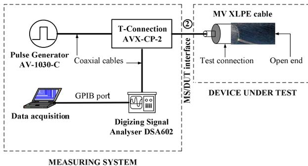
**Fig. 3.** Schematic drawing of the TDR measuring set-up [9]
