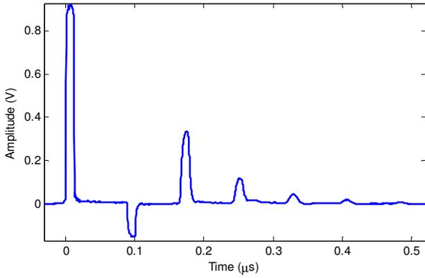
**Fig. 4.** TDR response when the DUT is open-circuited
