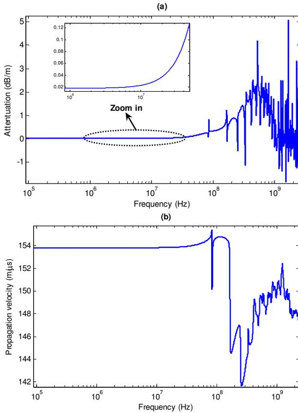
**Fig. 7.** Measured wave propagation characteristics of single-phase MV XLPE power cable; (a) attenuation constant, (b) and propagation velocity
