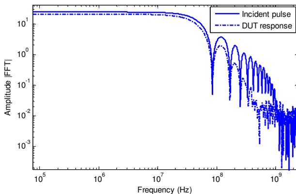
**Fig. 8.** FFTs of the incident pulse and the DUT response
