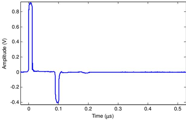
**Fig. 5.** TDR response when the coaxial cable 2 is short-circuited
