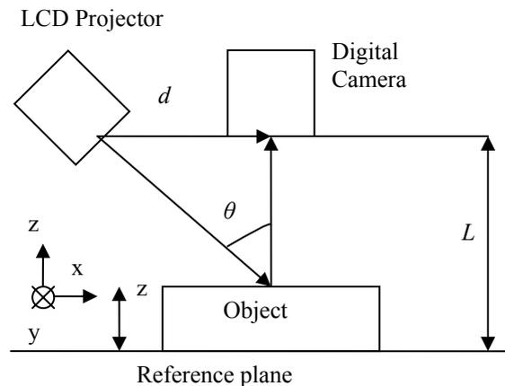
Figure 12. Fringe projection setup with LCD projector and digital camera.  $L$  is distance from pupil of the camera to the reference plane,  $d$  is distance between pupils of the camera and the projection.
