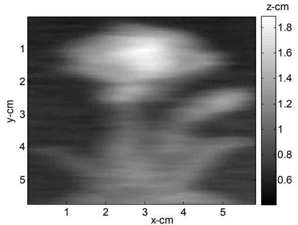
Figure 11. The profile of the object that is calculated by CWT phase algorithm for first setup.
