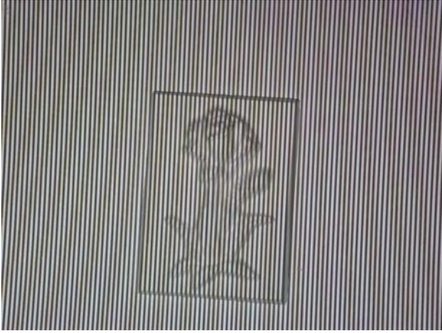
Figure 13. The object with fringe pattern that is reflected by LCD projector.
