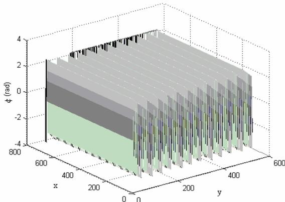
Figure 6. The wrap phase distributions of the inverse Fourier transform of the filtered simulated fringe pattern.
