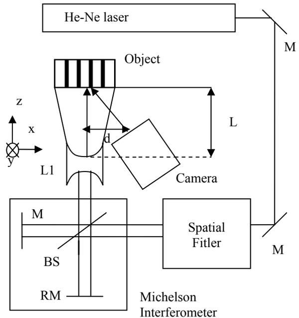
Figure 8. Fringe projection setup with michelson interferometer and CCD camera. M:Mirrors, RM:Reference mirror, BS:Beam splitter, L1: Lenses
