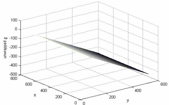
Figure 4. Unwrapped phase distribution of the CWT of the simulated fringe pattern.
