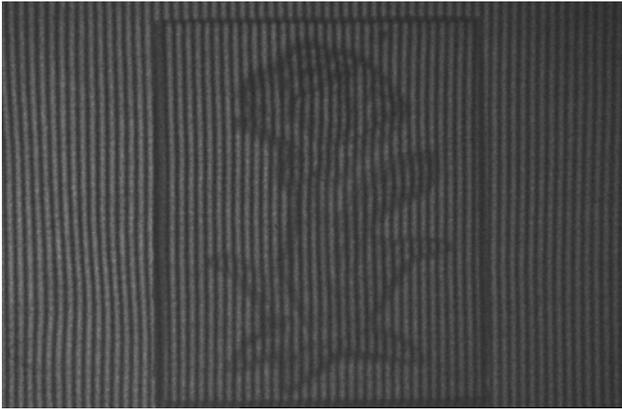
Figure 9. The object with fringe pattern that is produced by Michelson interferometer
