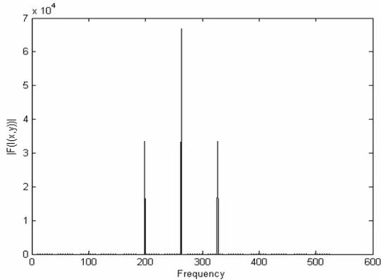
Figure 5. For one row the Fourier transform of the simulated fringe pattern.
