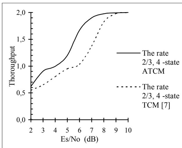
Figure 3. The lower bounds on the throughputs of HARQ using the rate 2/3 4-state asymmetric and symmetric TCM over an AWGN channel.
